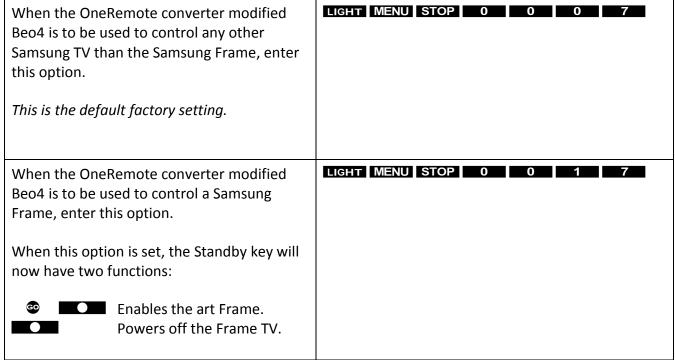
Simply, at any time, enter the corresponding 7-key sequence from the table to set the desired option on the OneRemote modified Beo4.
