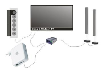
Add music to any Bang & Olufsen system wirelessly using Apple Airplay or Bluetooth or cable directly via the OneRemote PowerLink AUX Expander:
