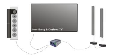
When the Bang & Olufsen radio is powered up, sound from the radio is automatically routed through the AUX Expander.
