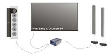
When the Bang & Olufsen radio is powered up, sound from the radio is automatically routed to the speakers.
