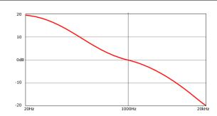
RIAA equalization is a form of pre-emphasis on recording and de-emphasis on playback. A recording is made with the low frequencies reduced and the high frequencies boosted, and on playback the opposite occurs. The net result is a flat frequency response, but with attenuation of high frequency noise such as hiss and clicks that arises from the recording medium.
