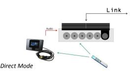
The CableLink option allows for the tuner to be listened to **and** controlled from any linkroom.
