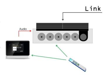
If the Bang & Olufsen system has no **AMEM** or **ATAPE** operated input available, the DabWiFI7 needs to be connected to a different input socket and reprogramming of the DabWiFI7 is required accordingly. **See the Installation Manual**.
