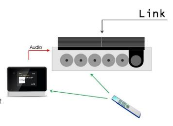
If the Bang & Olufsen system has no **AMEM** or **ATAPE** operated input available, the DabFmBlue5 needs to be connected to a different input socket and reprogramming of the DabFmBlue5 is required accordingly. **See the Installation Manual**.
