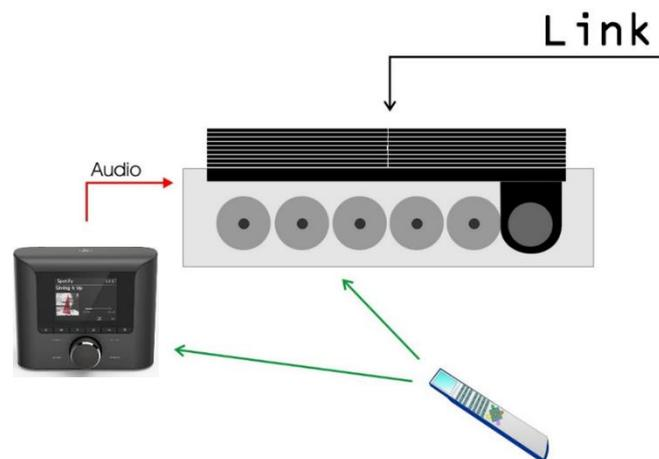
If the Bang & Olufsen system has no **AMEM** or **ATAPE** operated input available, the DabWiFi6 needs to be connected to a different input socket and reprogramming of the DabWiFi6 is required accordingly. **See the Installation Manual.**
