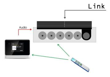
If the Bang & Olufsen system has no **AMEM** or **ATAPE** operated input available, the DabWiFi5 needs to be connected to a different input socket and reprogramming of the DabWiFi5 is required accordingly. **See the Installation Manual**.
