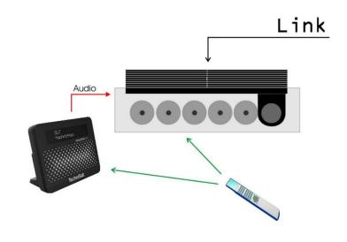
If the Bang & Olufsen system has no AMEM or ATAPE operated input available, the CableRadio1 can be connected to a different input socket and reprogramming of the CableRadio1 is required accordingly. See the chapter about Options.
